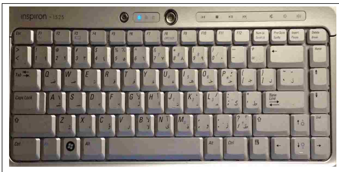
Figure 3-3 Our Arabic keyboard. On each key is marked two characters: an Arabic letter and a Roman letter.
